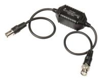
The GL001HDP Video Ground Loop Isolator is a passive devices which reduce Ground Loop Interference with HD CCTV signals and can easily install in a new or added to existing systems. It is useful where a video signal is transmitted via cable between points with different ground potentials, Differences in ground potentials are typically caused by unbalanced power line loads.
