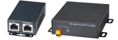
This IP06I90/IP06S60 are ultra high power POE 90W injector and full 60W POE splitter solution to send data and power over original Ethernet network but eliminates the need of power cable and converter. This adds POE functionality to non-POE devices whose power consumption is up to full 60W. It is perfect for network devices need higher power, such as IP PTZ speed dome camera, outdoor access points , touch PC, remote digital signage display...etc.
