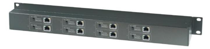
IPO8P Extender is designed to send and extend POE camera devices over existing coax cable. 8 Channel 1U rack panel type for professional and big system installation. The distance could up to 300 meters by RG6U  $75\Omega$  Coaxial Cable. They are completely transparent to protocols, codes, and applications ensuring compatibility with any POE camera and its management software. It is perfect solution to replace the analog camera to POE camera using existing coax cable.
